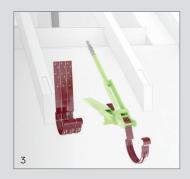
Before you mount the brackets (CJ), you should bend them so they match the angle of the roof inclination with a special device, according to the drainage slope.
