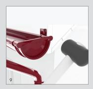
The universal stop (CU) end is fixed manually or using an elastic hammer at the end of the gutter, without using silicon because it destroys the gasket through time.
