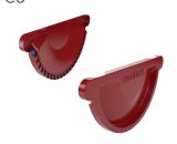
Is mounted onto the gutter on both ends Tightly sealed profile due to internal gasket Do not use silicone sealant, given it could lead to the deterioration of the gasket over time Pressed stop end for reinforcement
