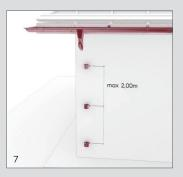
For the installation of downpipes (BU), attach the downpipe holders (BB) on the wall, one below the other, depending on the type of facade: in two side ears, central with a stud or vertical with poprivets. The maximum distance between two holders will not exceed 2 meters, while for each downpipe at least two support brackets will be used.
