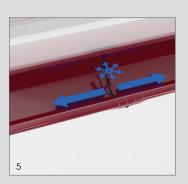
Two gutters that are to be joined should be placed on the brackets without being fixed. The distance between the edges of the gutters should be approximately 2-3 mm, as the The gutters and the corners (KEB / KIB) have the property to expand and contract according to the temperature variations.
