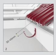
It is recommended to mount the gutter so that its outer side is 30-40 mm lower than the imaginary extension of the roof structure. Thus, the flow of water from the roof will not go over the gutter.
