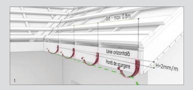
Before mounting the hooks, you should draw a drainage slope towards the place where you will place the pipes. It is preferable to make the slope of the gutter about 2 mm for each meter of its length. The distance between the hooks should not exceed 0.8 m, and the hooks at the ends should be placed 0,1 m from the edge of the roof.
